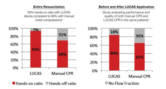
"Mechanical chest compressions provided by the LUCAS device improve CPR quality by significantly reducing the NFF (no flow fraction) and by improving the quality of chest compression compared to manual CPR during OHCA resuscitation."<sup>3</sup>
